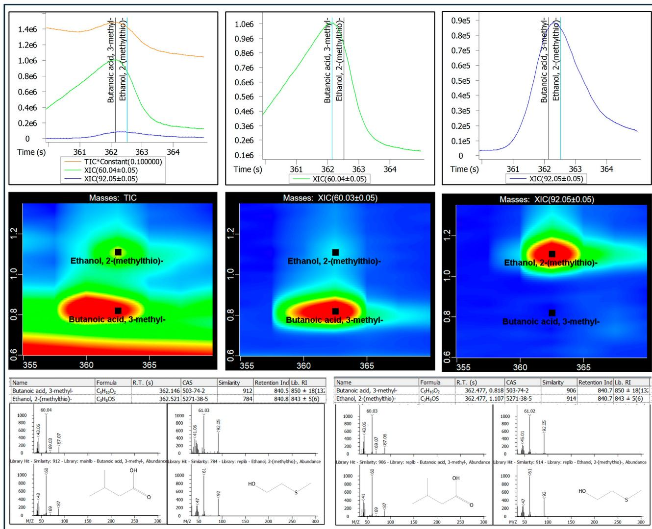
Figure 3. Some coelution pairs are deconvoluted with GC and chromatographically separated with GCxGC. Peak tables and spectral information are shown from the GC data (bottom left) and from the GCxGC data (bottom right).
