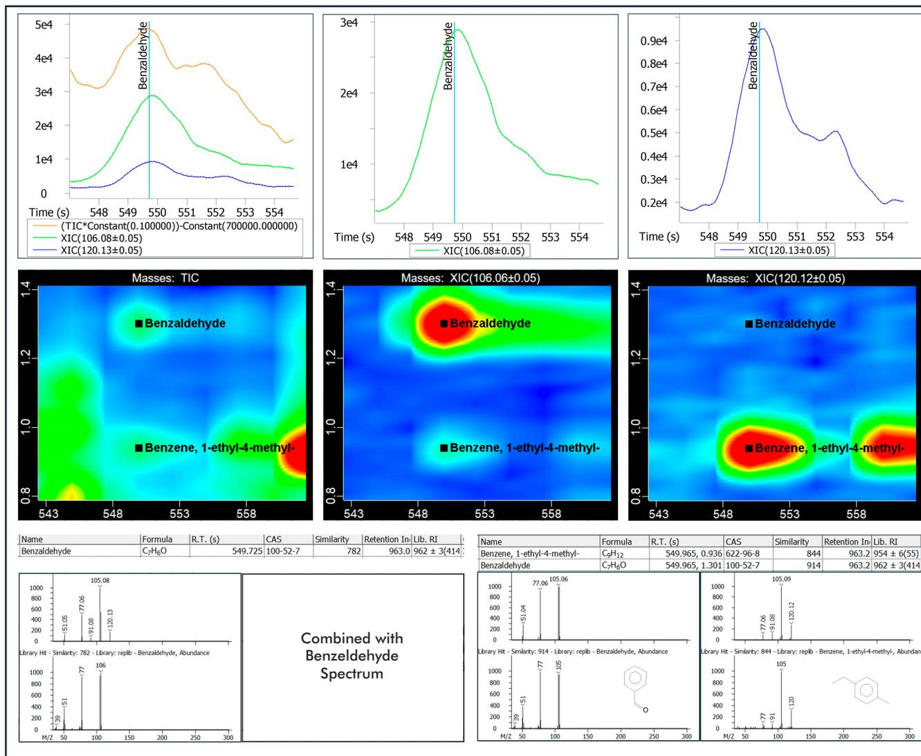
**Figure 4. Some coelution pairs exceeded deconvolution with GC and needed the additional peak capacity of GCxGC to be determined. Peak tables and spectral information are shown from the GC data (bottom left) and from the GCxGC data (bottom right).**
