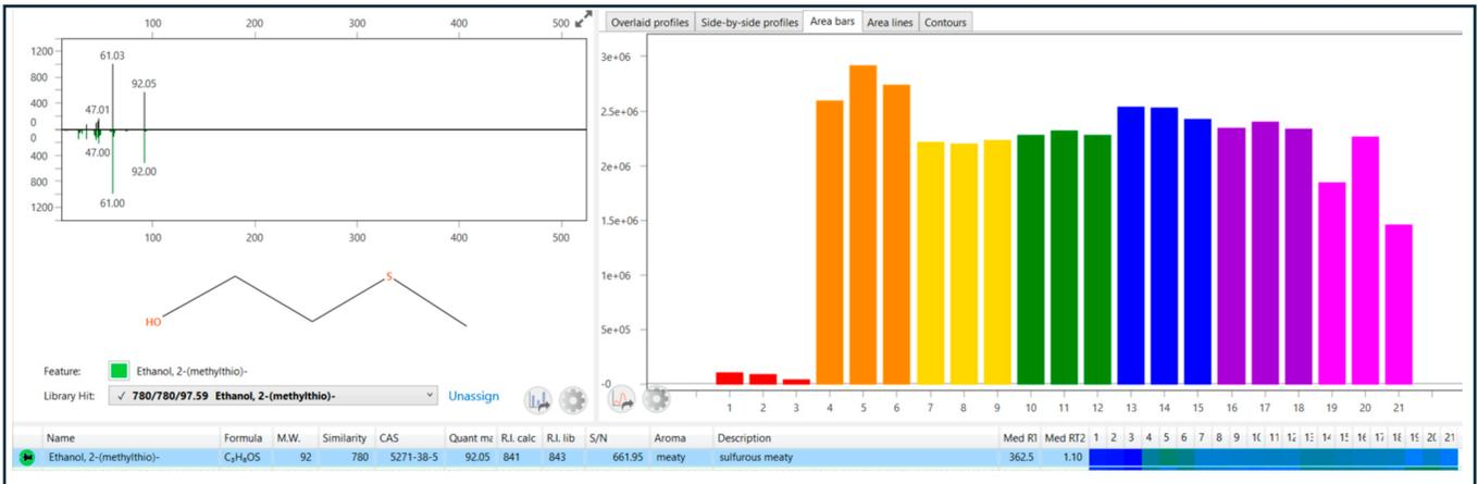
Figure 7. 2-(methylthio)-ethanol was determined in the food spoilage samples with Pegasus BTX 4D and ChromaTOF Sync 2D.
