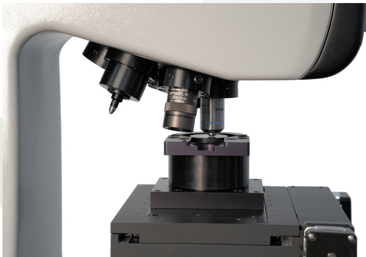
Six-position, angled turret design
