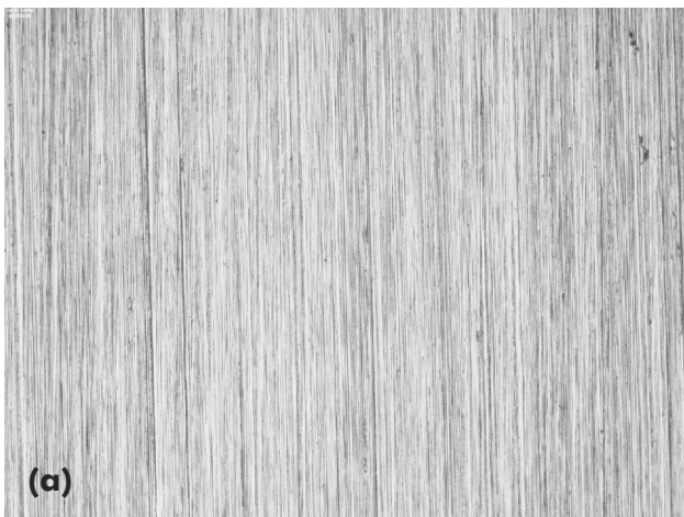
Figure 6: Carbon Steel Alloy Ground by (a) Manual Procedures and (b) Automatic Procedures 100X.
